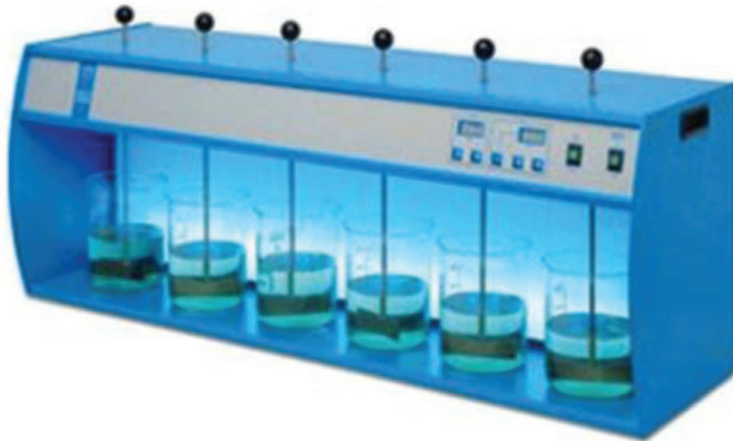
Figure 4.15 Typical Jar Testing apparatus
